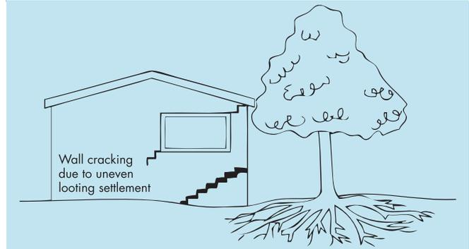
external footings. The doming is accentuated and cracking reduces or disappears where it occurred because of dishing, but other cracks open up. The roof lines may become convex.
