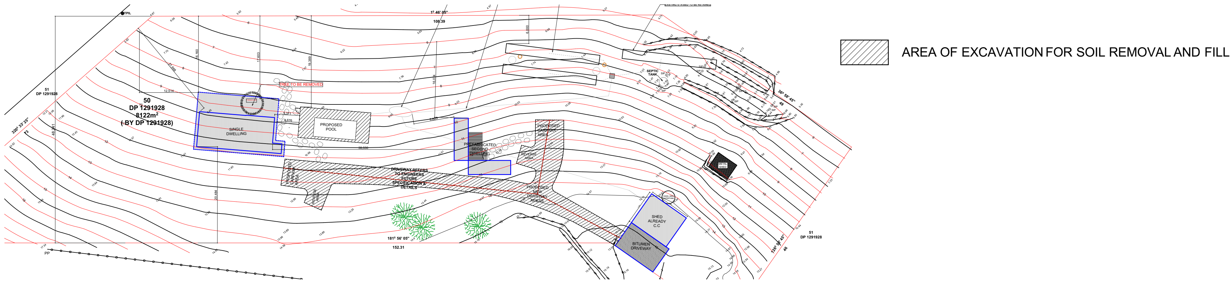
Proposed Excavation Work Plan Scale 1:500
