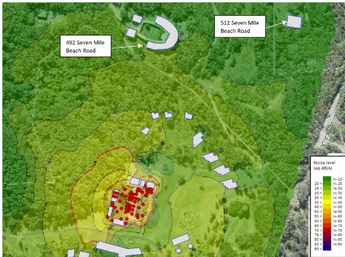
Figure 5.10: Patron usage of pool area – Lw of 65 dB(A) per point source – 35dB(A) limit line (Source: Greg Alderson and Associates, 2021).
