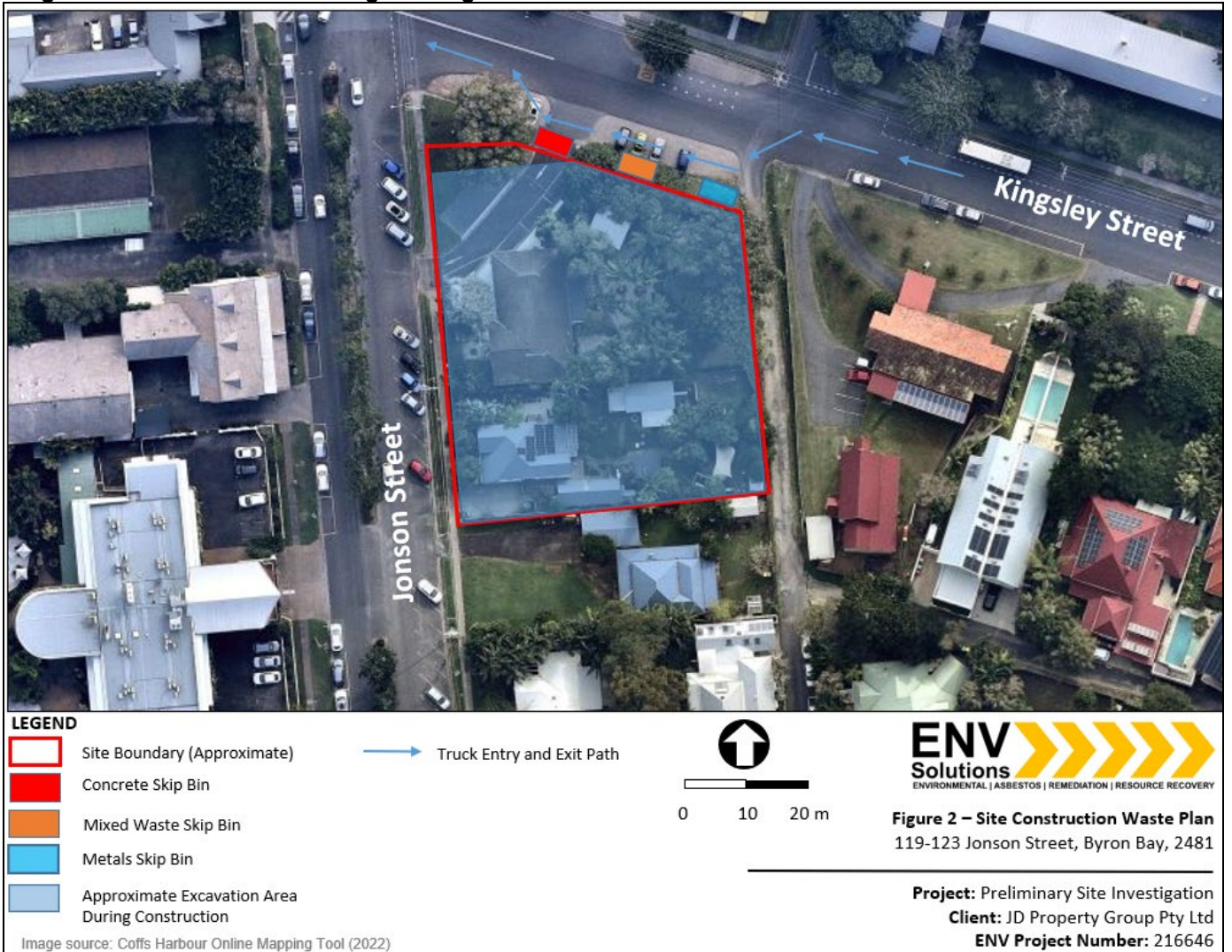
Figure 2: Location of Bin Storage During Construction
