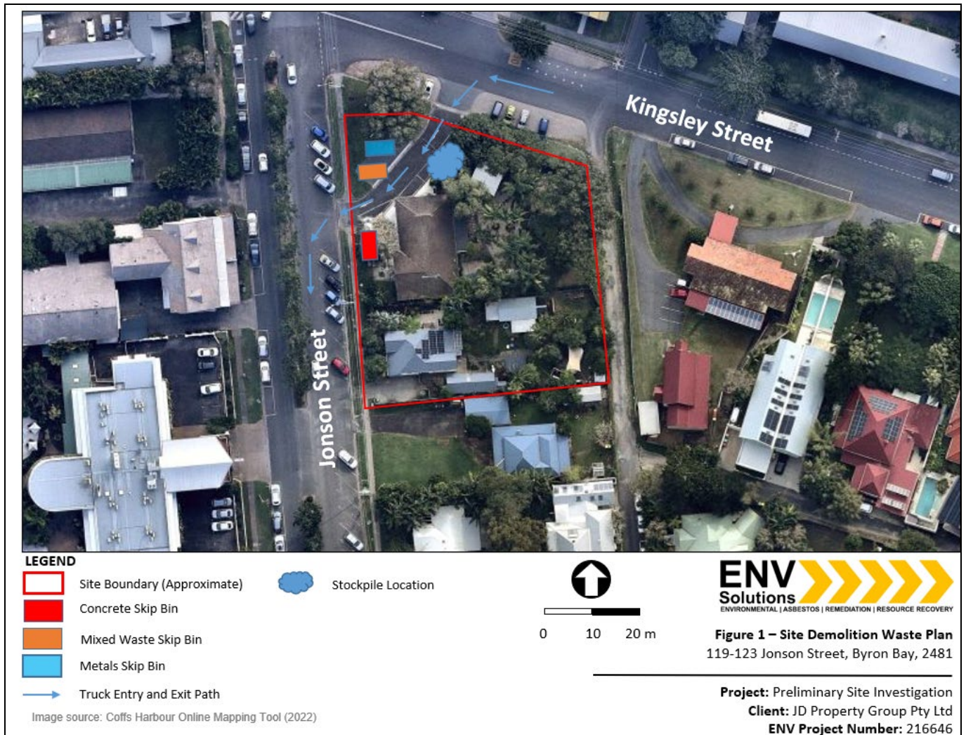
Figure 1: Location of Bin Storage During Demolition
