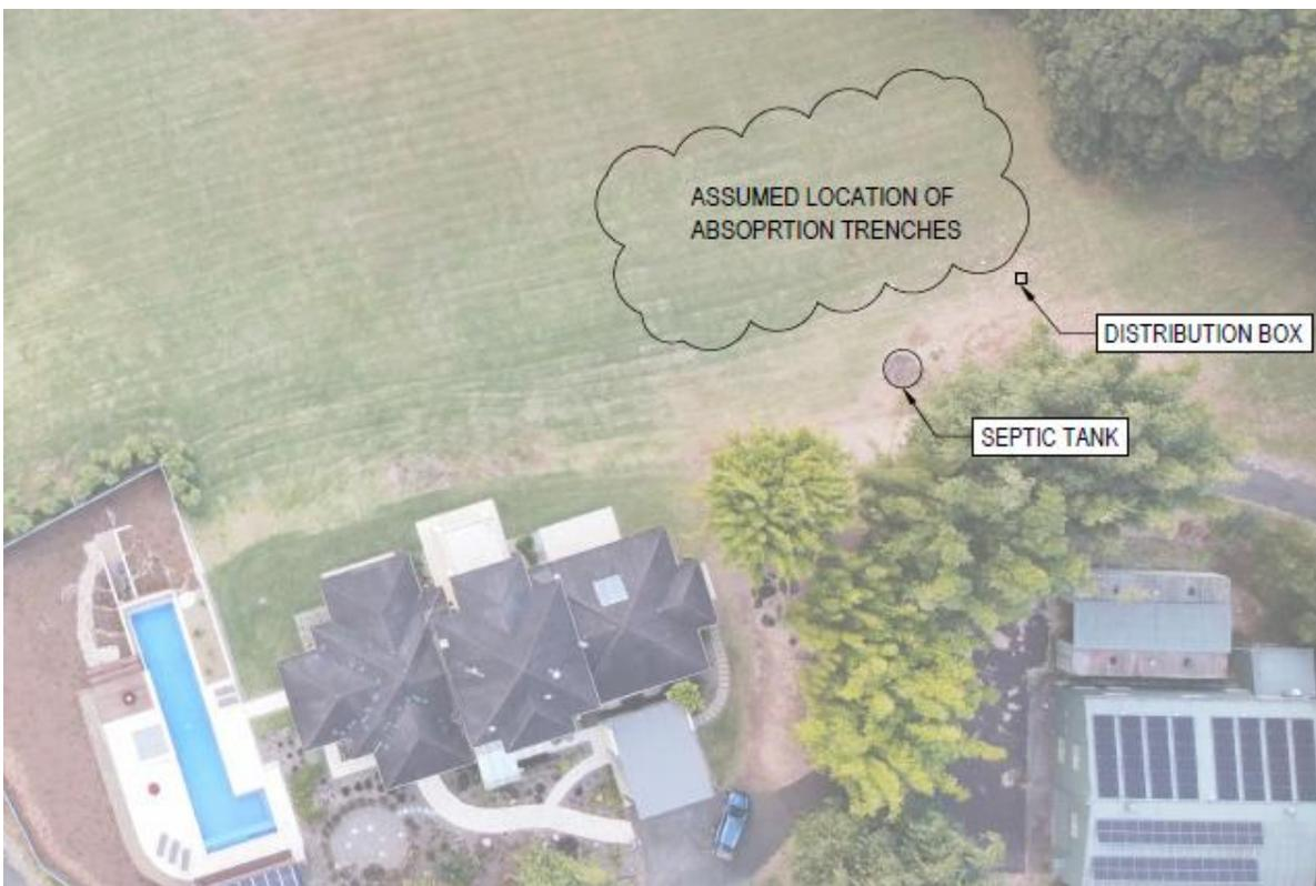
Figure 3 – Diagram of existing OSSM system (aerial image: NCWS 17.06.23)
