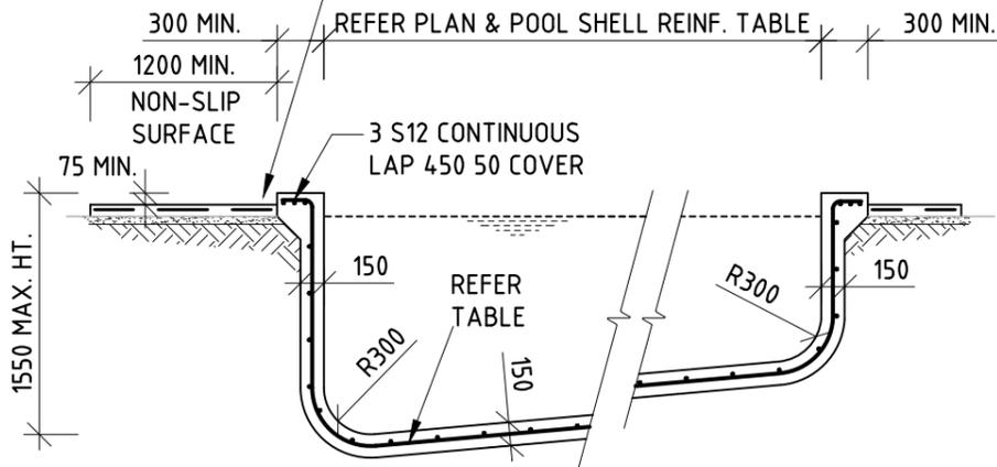
BASE OF SHELL TO BE COMPACTED TO 60% DENSITY INDEX & APPROVED BY INSPECTING ENGINEER
