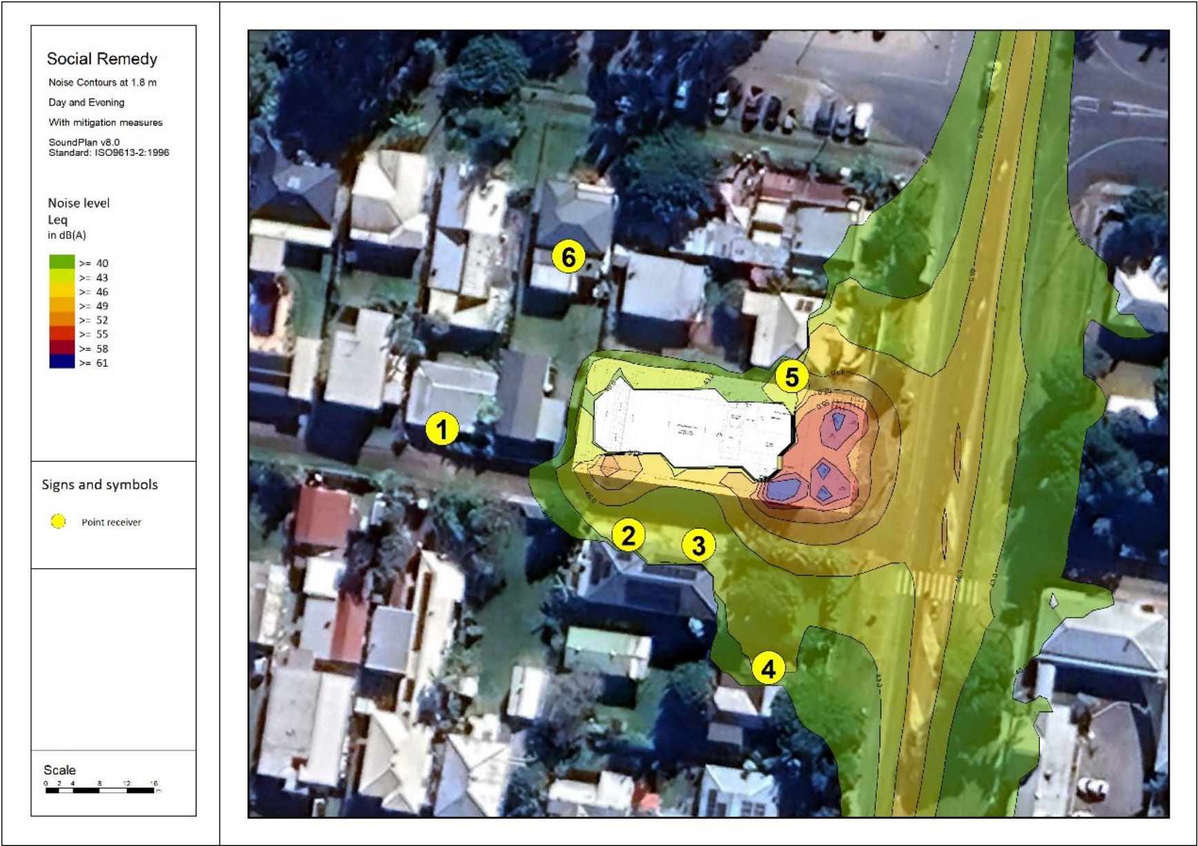
Plate 3.7 Noise contours at First Floor (4.6m above ground) with mitigation measures, day and evening noise sources. Levels are in dB(A) Leq
