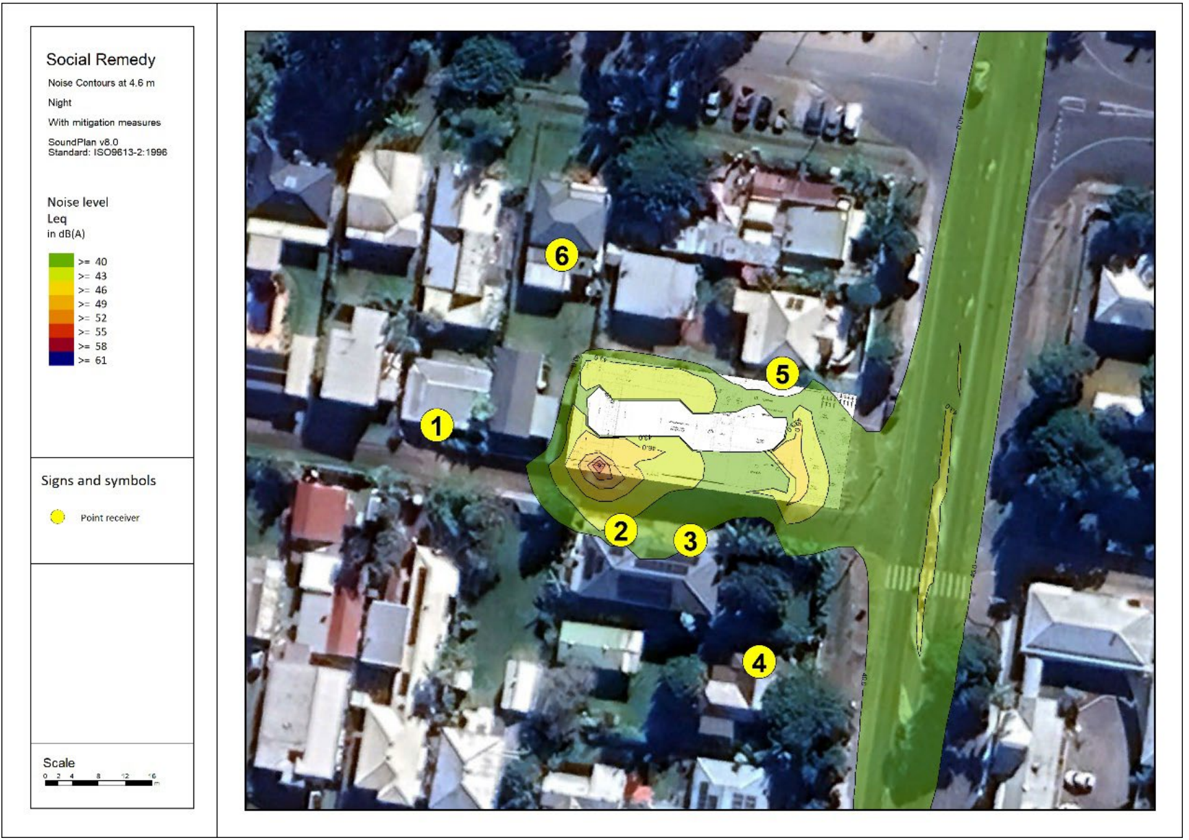
Plate 3.9 Noise contours at First Floor (4.6m above ground) with mitigation measures, night noise sources. Levels are in dB(A) Leq.
