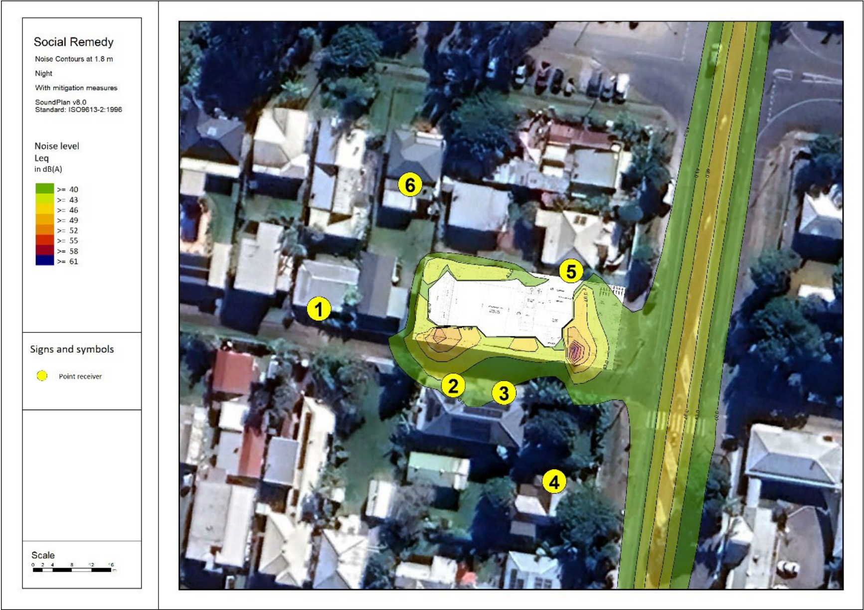
Plate 3.9 Noise contours at First Floor (4.6m above ground) with mitigation measures, night noise sources. Levels are in dB(A) Leq.
