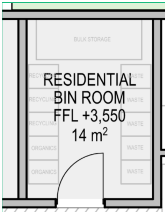
Figure 5-1 Residential Refuse Room
