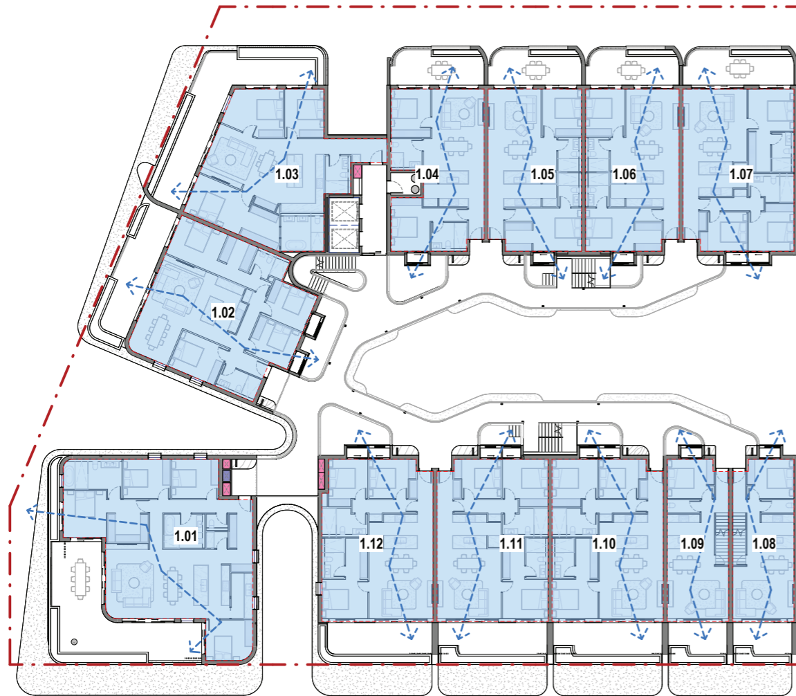
1 CROSS VENTILATION COMPLIANCE - LEVEL 01 DA201 1:200
